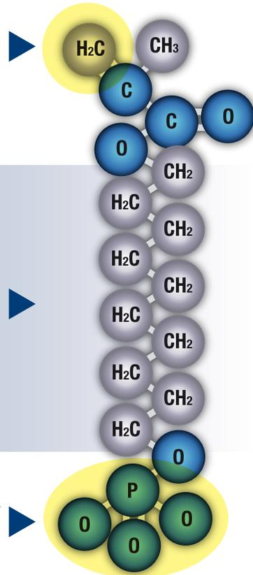
Long hydrocarbon chain results in a hydrophobic surface, and thereby modifies the interface to a water-resistant field.
