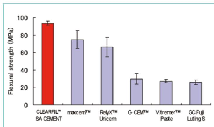
Figure 1. Flexural strength of self-adhesive resin cements. Adapted from H. Yamamoto, T. Nakamura, K. Wakabayashi, A. Okada, S. Kinuta, H. Yatani, Osaka University, 2008.
